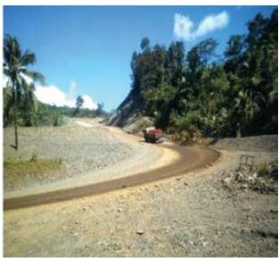
Dust is the prevalent problem in Nickel Laterite Mining. Laterite materials are so fine they become airborne during hot weather and turns into mud during rainy season.
